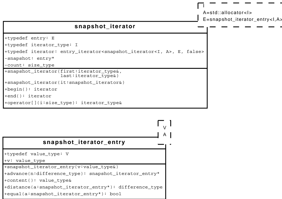
Figure 4. An overview of the snapshot iterator design
